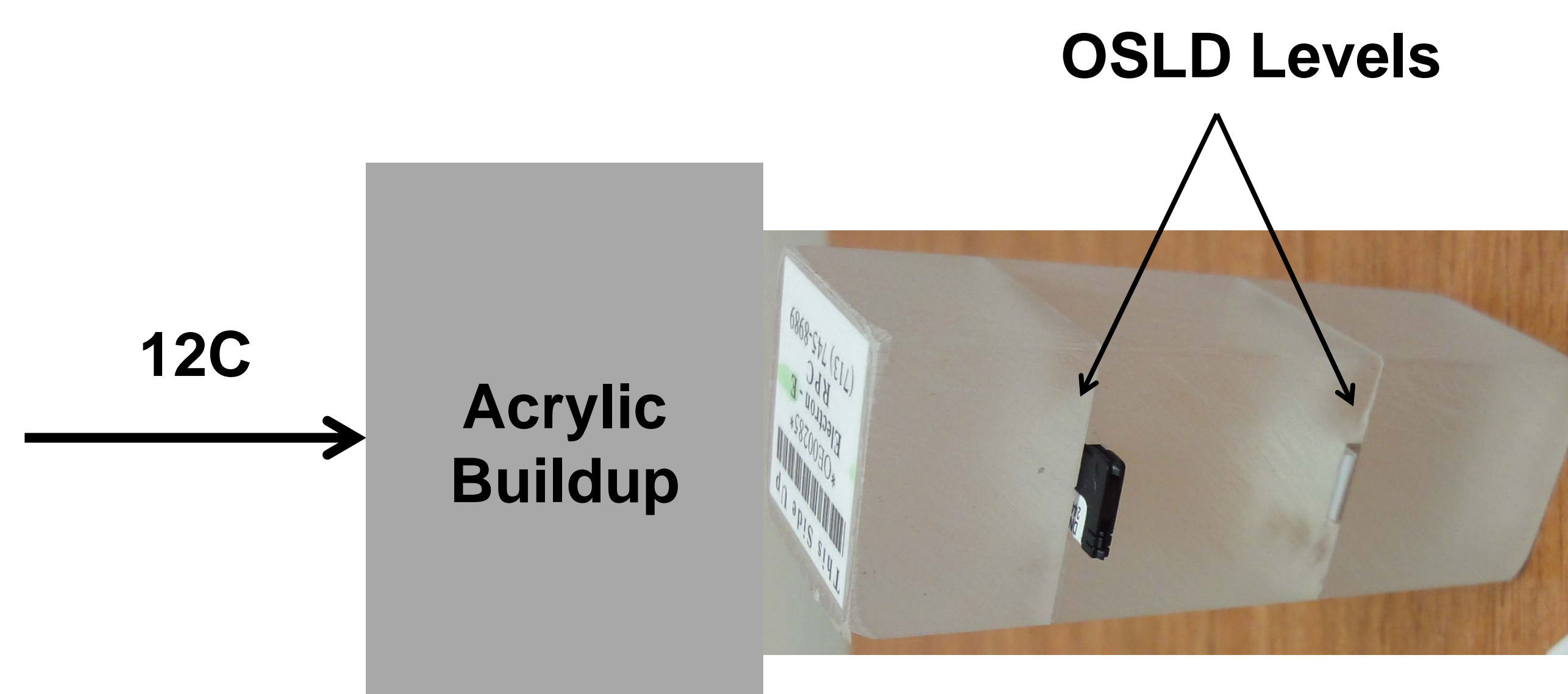
Figure 1. Setup for carbon OSLD irradiations, with variable acrylic buildup used for each maximum energy.
